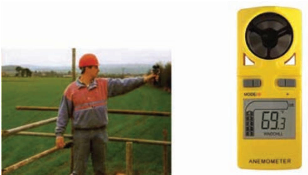
Figure 11.5: Using an anemometer to check wind speed at roof level.
