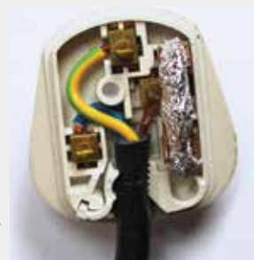
Dangerous electrical plug giving rise to risk of electrocution.
